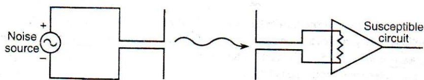
FIG. 6.8 Electromagnetic coupling. Radiated electromagnetic energy requires an antenna in both the noise and susceptible circuits. The antenna must be an appreciable portion of a wavelength, so such coupling is usually at high frequencies ( > 15 MHz).
